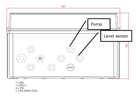
• Connect the level sensor and pump in the connection box as shown below.
